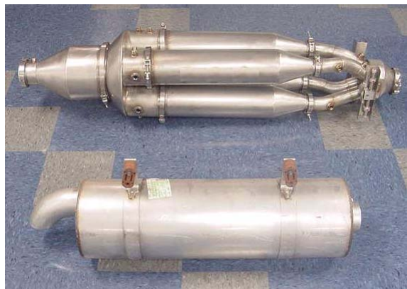
Figure 2. Size comparison of four-flow path system with a typical medium-heavy-duty diesel muffler. 31
