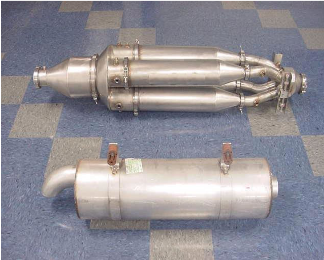
Figure 15. Comparing the Package Size of EPA's 4 Leg System to a Conventional Muffler
