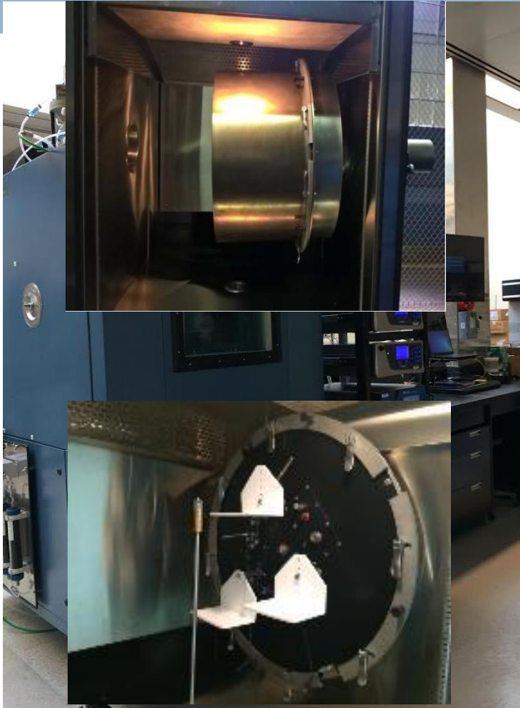
T and RH controlled : T (0-50 °C); RH (5-95%)
