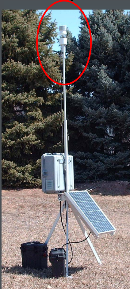
Latest version of the POMS II - - Sonic wind sensor plus ambient T and RH.
