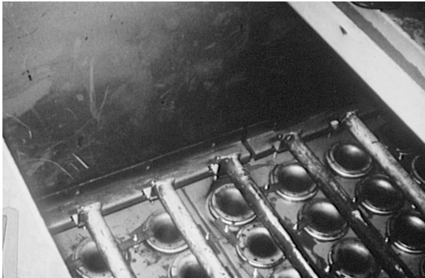
Figure 3-15. Clean side of a top access pulse jet baghouse
